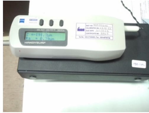
Fig.4 Handy surf E-MC-S24B for Surface Roughness Measurement
